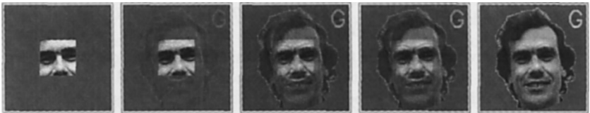
Figure 3.7 An example of the recognition of a face that was learned by the computer, including its family name encoded by a letter Note. The recognition process takes place in the presence of all the other learned patterns.
